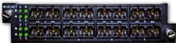
Duplex-Modul, 8x 100Base-FX, SC Monomode 1310 nm, 30 km
