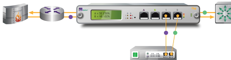
Figure 7: Half-duplex mode supports 100% utilization in both directions
