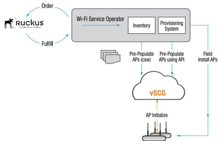
Figure 4: Automatic Access Point Configuration is the process by which APs installed in the field can have their configuration automatically downloaded to them via the vSCG.
